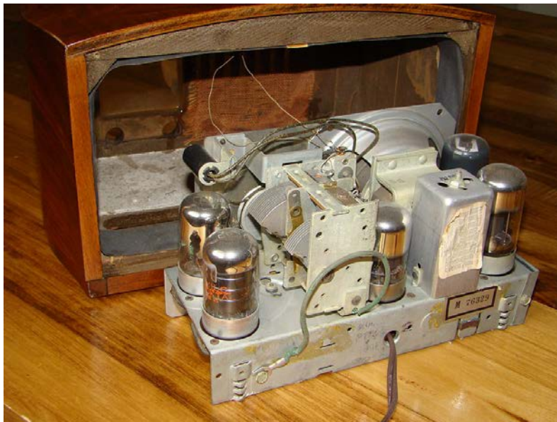
Figure 9 - Internal view of a “5 tube” superhet” table radio of Fig 7. Notice ganged variable capacitor towards the left, and the IF can towards the right.
